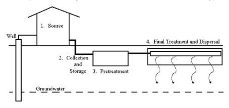
Components of an onsite wastewater treatment system.
